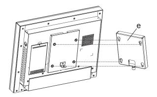
4. Fasten the thumb screw of the wall mount bracket (c) to fix the wall mount bracket (e) to the VESA bracket (a).
