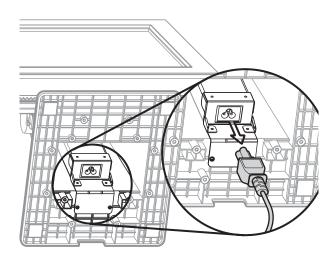
**2.** Unscrew the screws (x2) and separate the power bracket from the stand.
