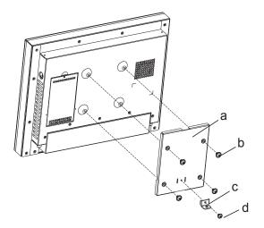
3. Align the tear drop holes of the wall mount bracket (e) into the 4 VESA bracket screws.
