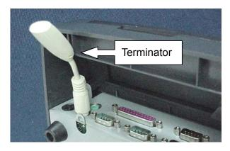
b. If you select K/B Wedge MCR, we provide a Terminator for you to insert into K/B PS2 for simulate PS2 K/B so you can use K/B Wedge MCR under NT/2K/XP OS.
