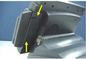
a. Push into the MCR module at the right side of System LCD Module then lock it with two screws.
