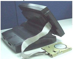
a. Connect the FDD cable from 40 pin FDD connector left side of LCD module..
