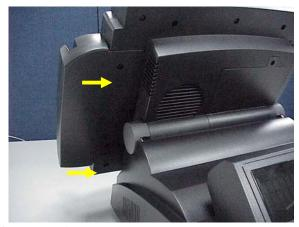
Push into the MCR module at the right side of System LCD Module then lock it with two screws.
