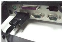
a. Insert the RS232 cable into b. Insert the other end of the any of the Com ports. b. Insert the other end of the RS232 cable into the RJ45
