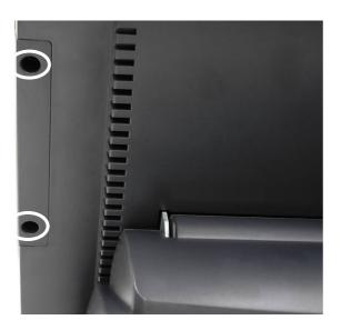
a. Remove the screws (2) of the plastic cover on the right side of the display.
