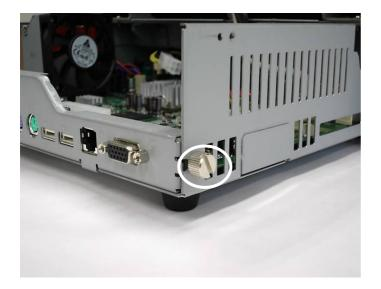
b. Disconnect the cables(3) as shown in the picture.
