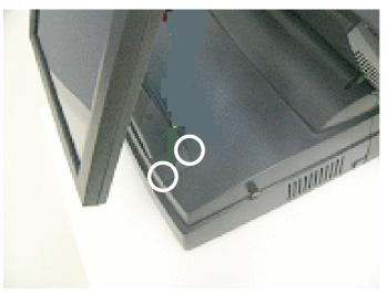
b. Mount the second display on the rear of the system and tighten the screws (5) on the supporter.
