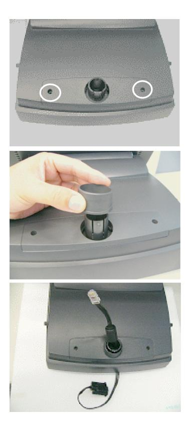
g. Install the VFD cover and tighten it with the screws (2).
