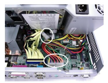
a. Disconnect the cables(2) as shown in the picture.
