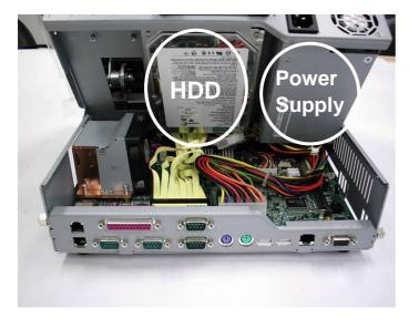
c. Pull the chassis box cover towards you by the handle, and lift it up.
