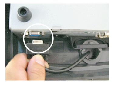
c. Insert the other end of the VGA cable (male) into the VGA port of the system to establish the connection.
