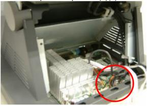
b. Disconnect the cables (5). IDE, LVDS, Inverter cable, touch cable, VFD cable
