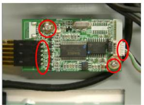
e. Remove the screws (2) and disconnect the cables(2).
