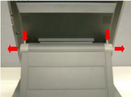
a. Press and pull to remove the hinge covers(2)
