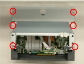
e. Remove the screws (6) to release the metal cover from the stand base
