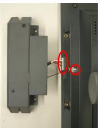
b. Connect the MSR cable (1) and secure the grounding cable with screw (1).
