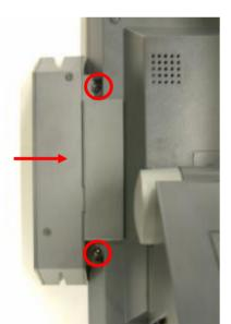
c. Place the MSR into the position and tighten the screws (2).
