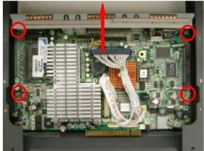
g. Remove the screws(4), and slide the mainboard in the direction as shown by the arrow.
