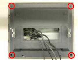
c. Remove the screws(4) and separate the back cover from the display head.
