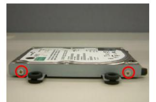
c. Remove the screws (4) to release the HDD d. Remove the screws(4) (two from each side) to release the HDD holders(2) from the HDD
