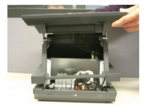
d. Lift the stand cover up to separate it from the stand base
