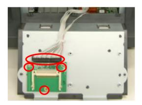
b. Disconnect the IDE cable and remove the screws(3) to replace the CF card holder.
