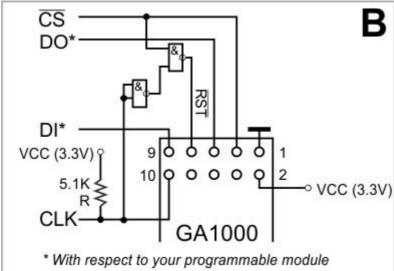
Tibbo devices differ in whether the CS, CLK, DI, and DO lines are remappable. On the  $\underline{\mathsf{EM1000}}$ ,  $\underline{\mathsf{EM1202}}$ , and  $\underline{\mathsf{EM1206}}$ , you can choose any set of GPIOs to control the GA1000. On the  $\underline{\mathsf{EM500}}$  where remapping isn't provided, you just have to use "prescribed" GPIO lines.
